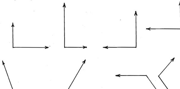
Carefully construct the vertical and horizontal components of the eight vectors.
