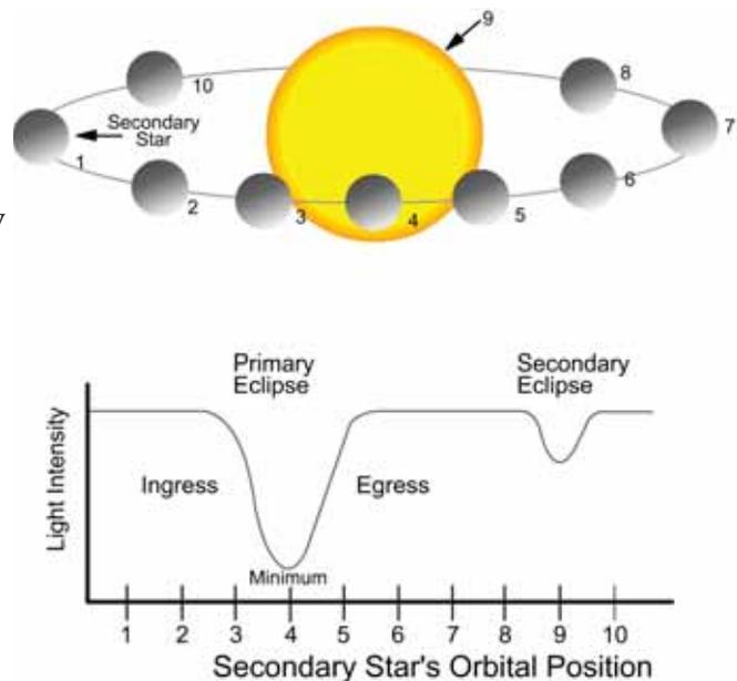
**Figure 3-5: Diagram and light curve of an eclipsing binary star system. Notice that the greatest change of light occurs when the orbiting star passes in front of its larger partner.**
