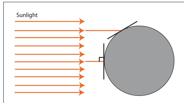
**Figure 1-20:** Diagram showing the angles at which sunlight reaches a world's surface. A world without an atmosphere or with only a very thin atmosphere will be hotter at the location where the sunlight is coming straight down, at a right angle to the surface, than at the locations where the sunlight is reaching the surface at a lower angle.
