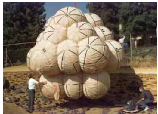
Figure 1-15: Photograph of airbags similar to those used by Pathfinder to land on Mars
