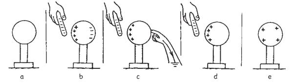
The diagrams below show a similar procedure with a positive rod. Draw the correct charges in the diagrams.
